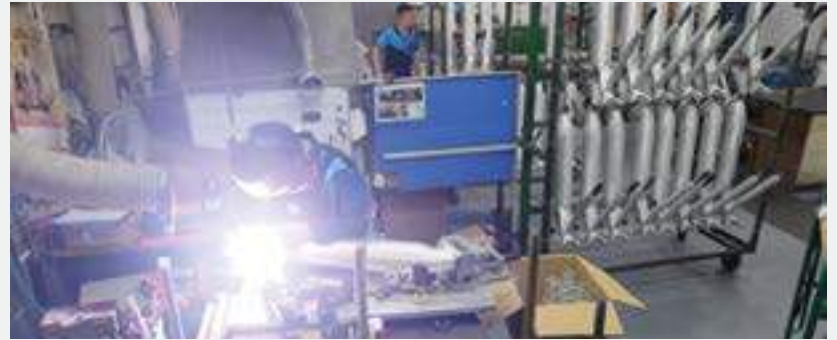
Due to its full focus on aluminum frames and forks, craftsmanship can be witnessed in action at Genio Bikes.
