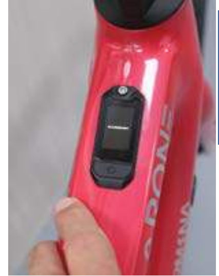
The display of the HX 200 system is neatly embedded in the toptube, adding to the unit's low-profile looks.
