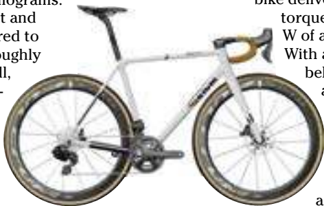
Cinelli's Speciale Corsa XCR blends Columbus stainless steel tubing with 3D-printed lugs and modern race standards.
