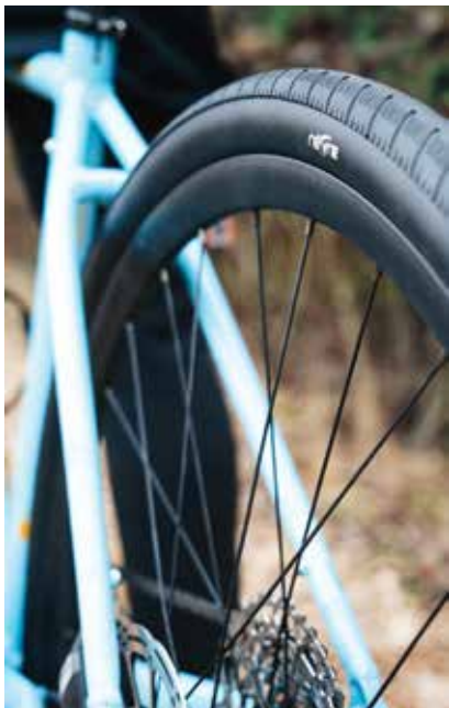
The Leka is a rubber-free tire made from 100 percent reusable materials.
