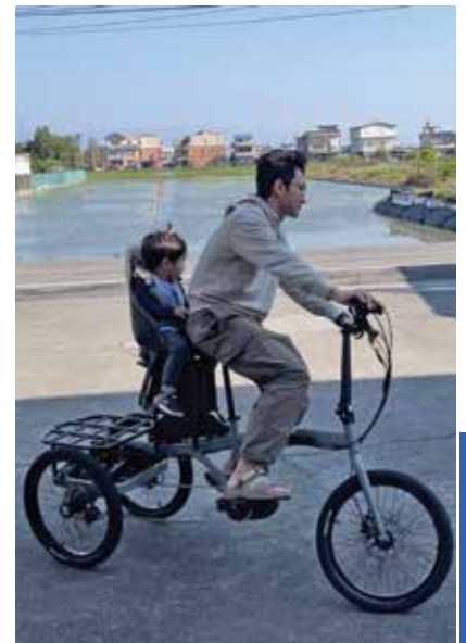
Naro Delta's leaning control system can be locked out for stability
