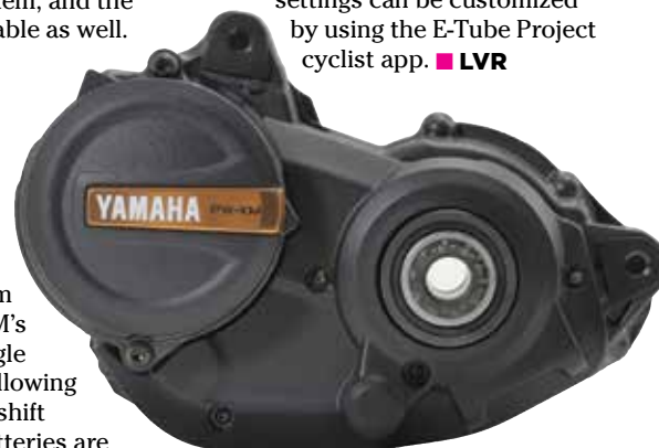
Yamaha shaved significant weight from its PW-XM flagship mid-motor with a magnesium housing.
