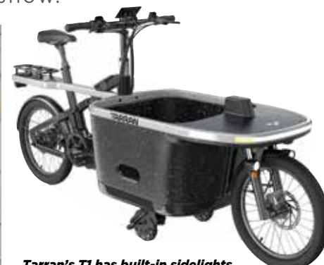
Tarran's T1 has built-in sidelights, cameras and a radar system for safety.
