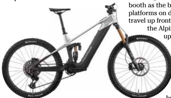
The Tarok Ultra of Raymon Bicycles relies on ZF's new compact CentriX e-drive system.
