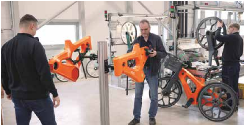
The Igus RCYL is a bicycle that is 50% made from recycled fishing nets.
