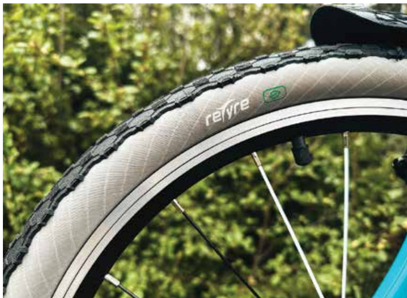
reTyre has developed a way to produce pneumatic tyres without the use of rubber.
