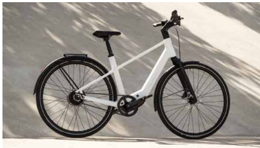
The Advanced Reco Urban is an e-bike based on a frame made from a special plastic injection moulding process.
