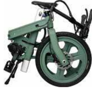
The DKCity db5 features mag wheels and a seatpost battery
