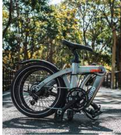
Oullon's E16-T6 uses a deflection rotation joint instead of a hinge for its main fold
