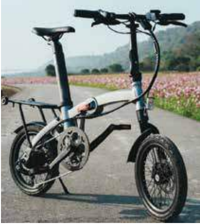
Oullon's E16-T6 uses a deflection rotation joint instead of a hinge for its main fold
