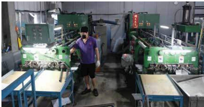
This workstation transforms straight-gauge titanium tubes into butted and swaged tubes
