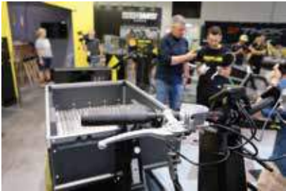
Disc brake systems for large cargo bikes come with a lot of motorbike technology.
