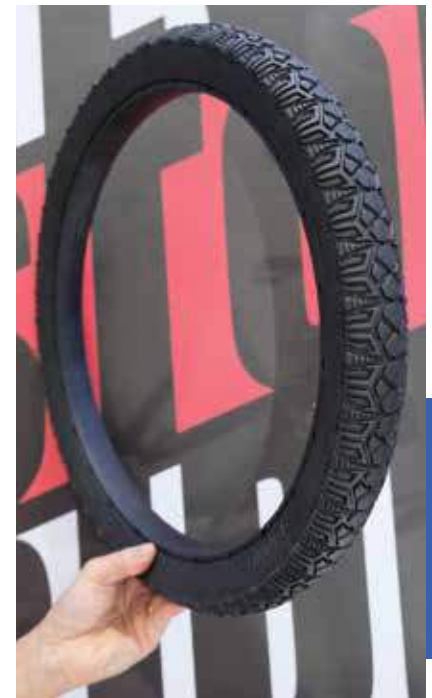
Since there's no air that could escape, the airless tires of Tannus are a welcome add-on for professional logistics.
