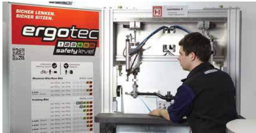
Humpert tests its parts stringently to classify them by safety levels.
