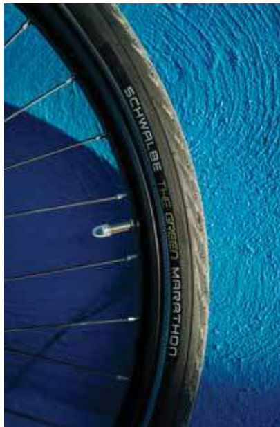
Schwalbe's Green Marathon has been updated and now contains 80% recycled and renewable materials.
