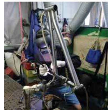
Ti frame welding demands a lot of expertise
