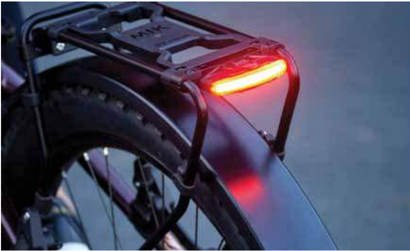
The Halo light from Spanninga features organic lines and integrated Z-reflectors
