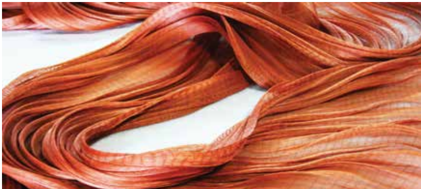
Formosa Taffeta's Etycord is a tyre cord material that is made out of recycled nylon fibres.
