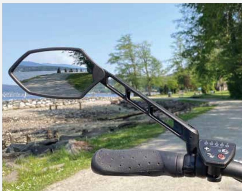
Unveiled at Taichung Bike Week, the mirror arm of the HF-M6002LSR052 is specifically designed to reduce weight and improve wind resistance, and the body is made of fiber-reinforced plastic.
