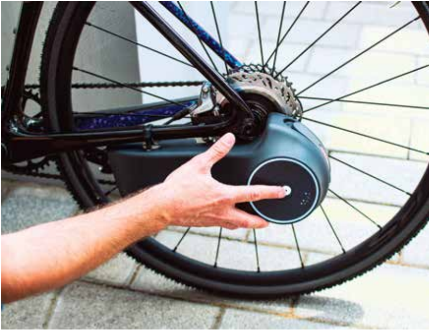
The "Disc Drive" kit from British company Skarper converts a conventional bicycle into an e-bike easily.
