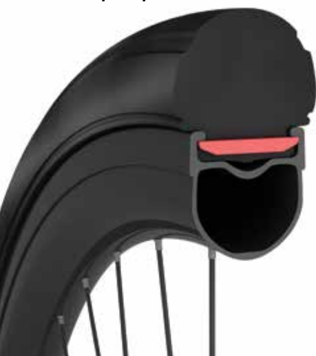
The Tannus airless tyre fits into a standard rim with special pins
