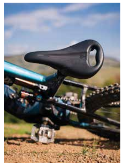
The prominent cut-out on WTB's Devo e-bike saddle helps when manoeuvring the bike.
