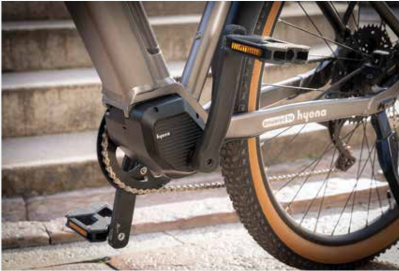
Hyena E-Bike Systems unveils its first mid-drive motor, the UniDrive 70.
