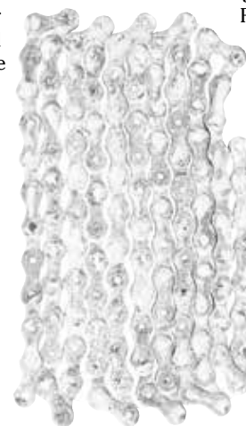
CeramicSpeed takes other makers' chains and treats them to reduce drag
