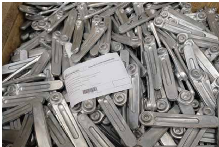
Forged aluminum crankarms await further processing.
