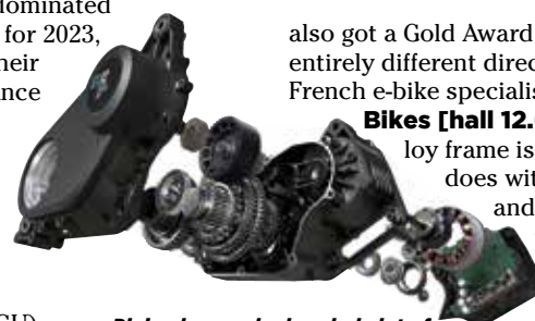
Pinion has packed a whole lot of technology into its motor and gearbox unit – and won a Gold Award with it.
