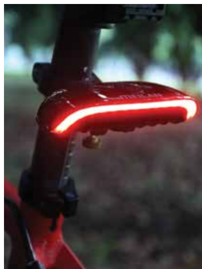
Mellan's Cute Eye offers indicators, a brake light, and added lasers
