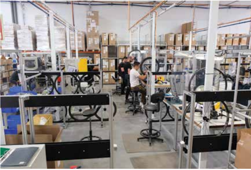
Assembly of Zipp wheels at Sram Portugal is mostly done by hand.
