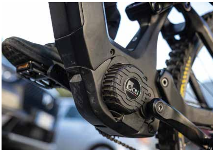
Thanks to their position in the bottom bracket, mid-motors have little impact on a bike's handling.
