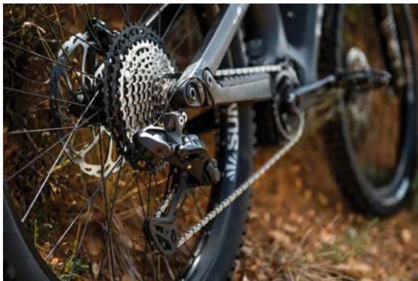
Shimano syncs the electronic shifting of its XT Di2 and Cues Di2 drivetrains with its mid-motors
