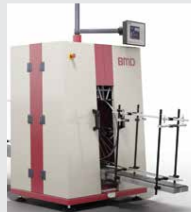
With modern technology, BMD's truing machine has a production speed of 40 to 100 wheels per hour.
