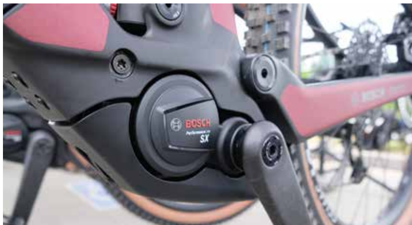
Bosch's most compact and lightweight mid-motor, the Performance Line SX, still packs a punch.
