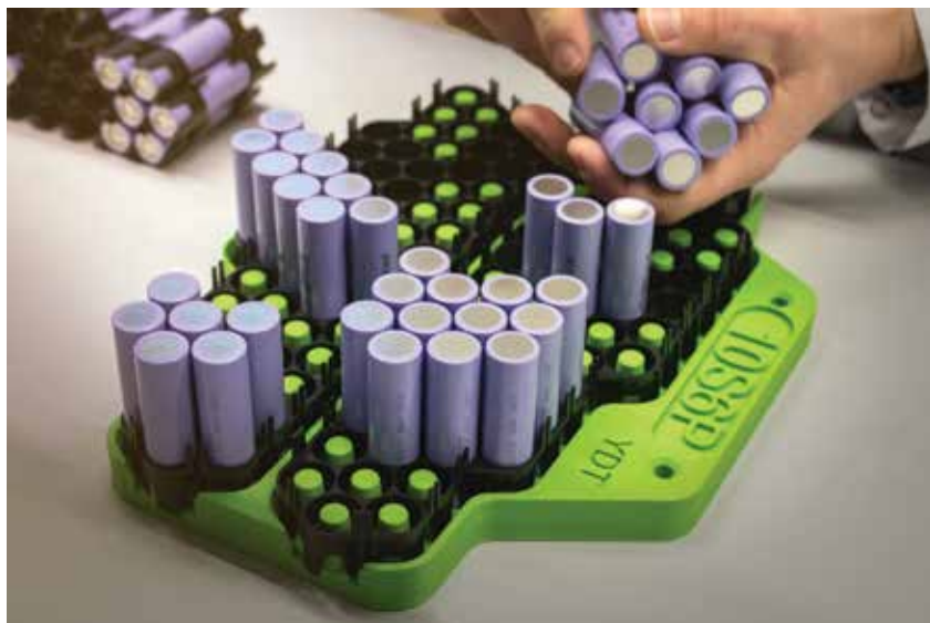
To make sure each battery is assembled correctly, the single cells are mounted in specific frames.
