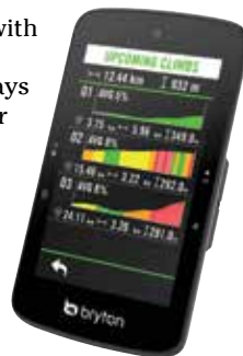
The Climb Challenge screen on the Bryton Rider S800 gives details of upcoming climbs
