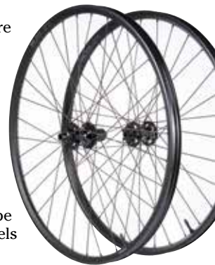
Seido's Magnon wheels can take a load of up to 150kg
