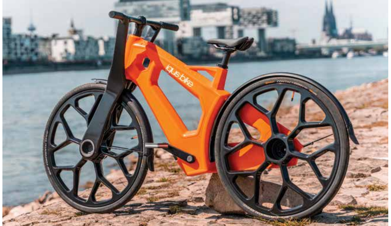
Fully made of plastic, the Igus:bike has no parts prone to rust and can be recycled at the end of its lifecycle. (photo: Igus GmbH)
