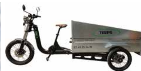
The Pick Up model of French manufacturer Trips has a tilting cargo bay.
