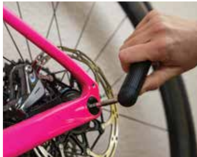
Locking into a T or an L shape, the Groove Pro tool from Ryder Innovation offers leverage and length beyond that of most multitools
