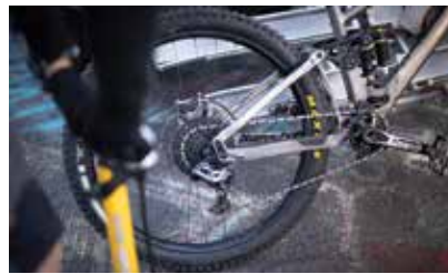
Stan's NoTubes Flow Mk4 wheelset uses M-Pulse hubs with magnetic freehub engagement
