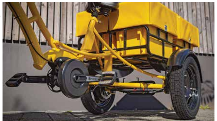
Without a chain or belt drive, the eDrive IN system of Pendix is ideal for heavy cargo trikes.
