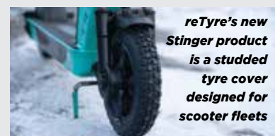
The reTyre system allows riders to adjust their tyre tread for the conditions without removing the wheels
