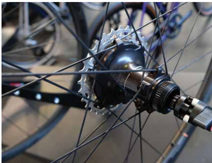
Classified's Powershift system replaces the front derailleur with a two-gear hub.
