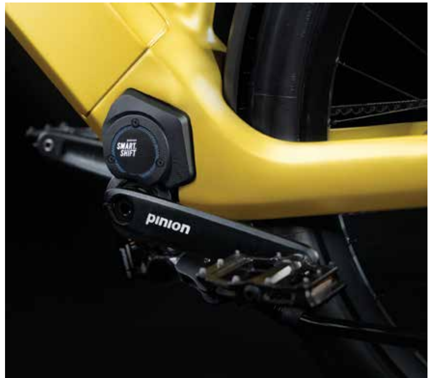
With the Smart Shift technology, Pinion has electrified its gearbox.
