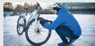
The reTyre system allows riders to adjust their tyre tread for the conditions without removing the wheels
