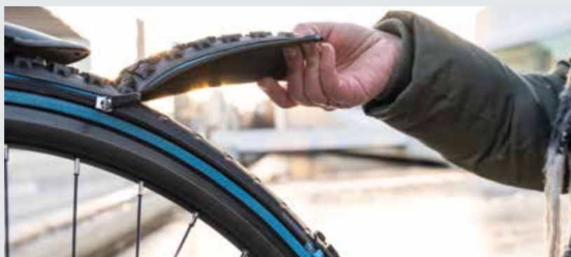
reTyre's modular system for bikes consists of a slick base tyre and a selection of treaded skins which can be zipped into place
