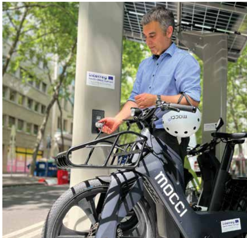
Hannes Neupert uses a LEV parking and charging location that conforms to the IEC TS 61851-3-Series Standard. The MOCCI Pedelec with innovative structure and drive system and be seen at Eurobike at the eFlow Europe booth (Hall 8.0 / E21).
