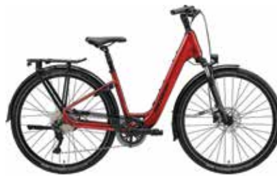
The eSPEEDER 400 EQ from Merida uses Mahle's popular ebikemotion X35 motor
