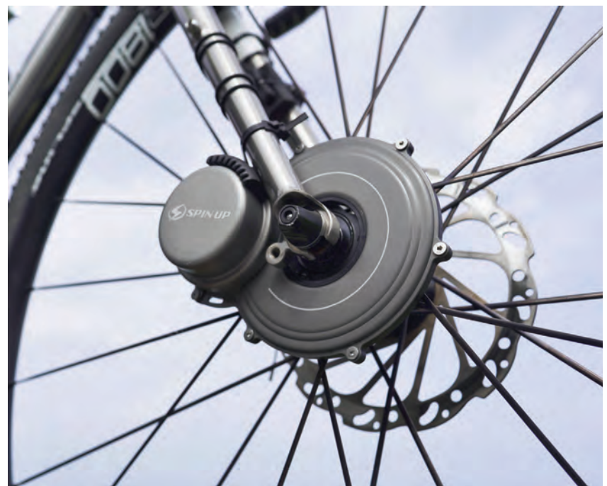
Spin Up's 1,000mA dynamo-based USB charger
