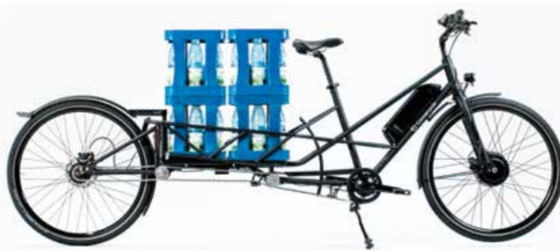
Convercycle: transforms from an ordinary bicycle to a cargo bike and back without tools
