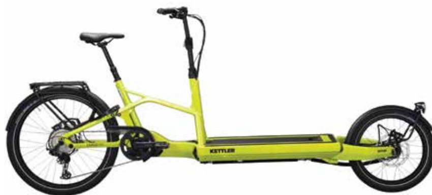
Kettler Cargoline series with Ackerman steering
