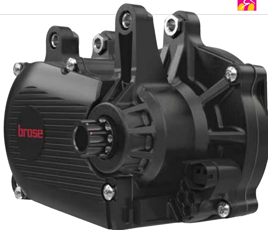
Brose is offering its Drive TF mid-motor in a magnesium housing
