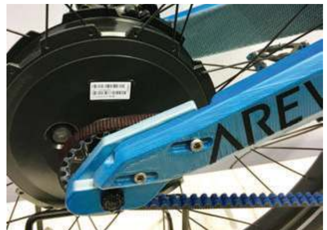
The EVE9 incorporates a Neodrives rear hub drive.
