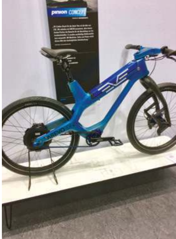
The prototype of the EVE9, at the Pinion booth, was made from a plastic composite. Arevo, its manufacturer, is preparing to produce a carbon fiber version for production that's made by a 3D printing process.
