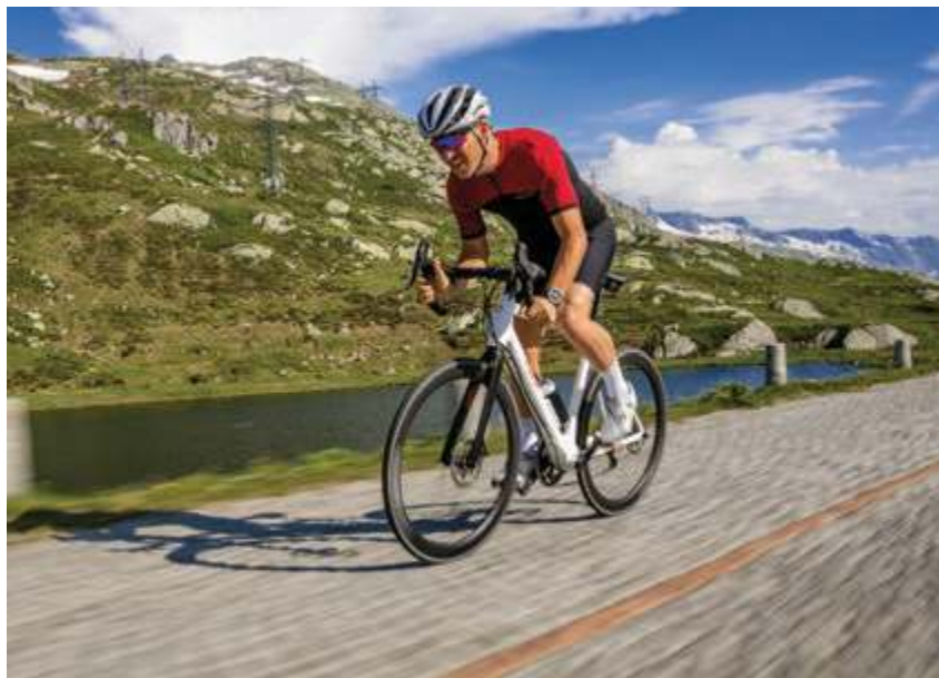
Maxon's e-road bike drive system in action. The "bottle" is the battery.
