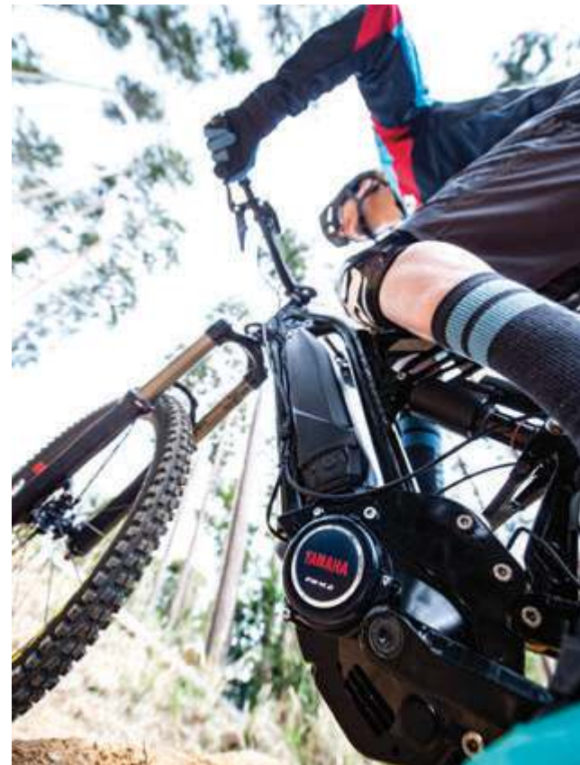
Yamaha's new PW-X 2 drive incorporates a fourth sensor that measures the incline of the terrain.
