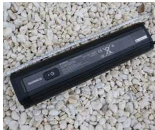
Shimano shrank the dimensions of its 504Wh integrated battery so it fits more easily into the downtube.
