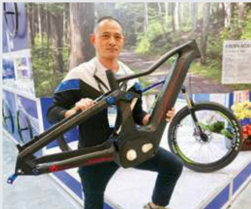
A-Pro COO Wayne Yang with a carbon and aluminum frame for a 29-inch, fully integrated e-mountain bike. (Photo by Jo Beckendorff)
