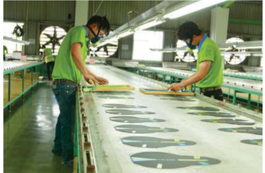
DDK workers use screen printing for graphics on new saddles.
