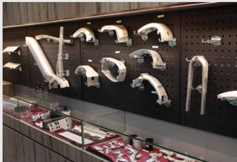
A selection of hydroformed e-bike parts on display at the A-Forge headquarters.
