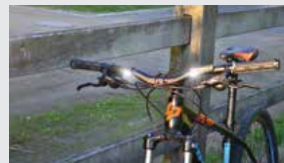
The Wink "smart handlebar" includes integrated LED lights, an associated app and an NFC hardware switch
