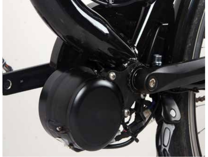
A mid-drive pedelec conversion kit (Photo: zedler.de)
