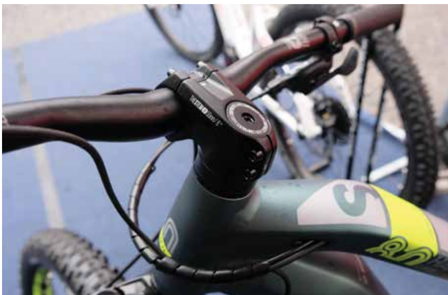
A bigger diameter adds to the stiffness and strength of Haibike's 'the Stem'.
