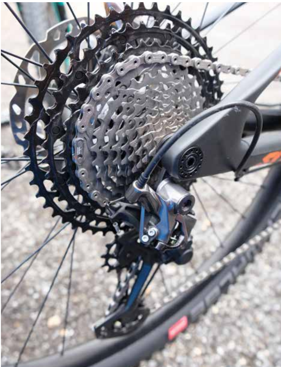
With fewer chainrings, the cogs grow in size - as with Shimano's new XTR.
