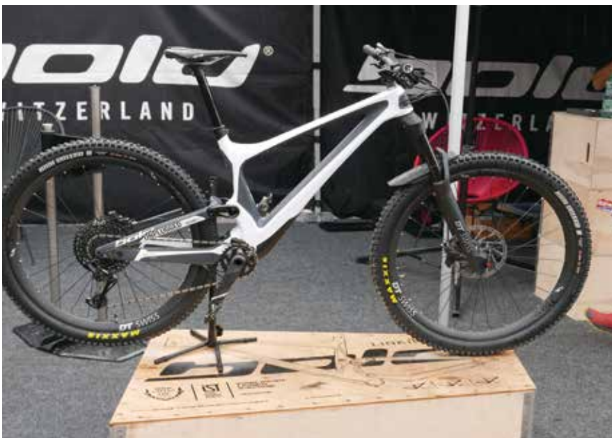
Clean look: Bold Cycles' new model 'Unplugged' with hidden rear shock and new F535 Fork from DT Swiss.
