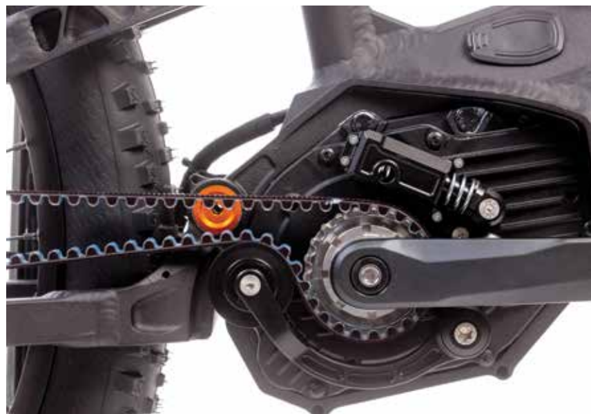
Close-up of the HNF Nicolai G16 Eboxx showing the belt tensioner behind the crank, enabling the full suspension bike to work with a Gates belt drive
