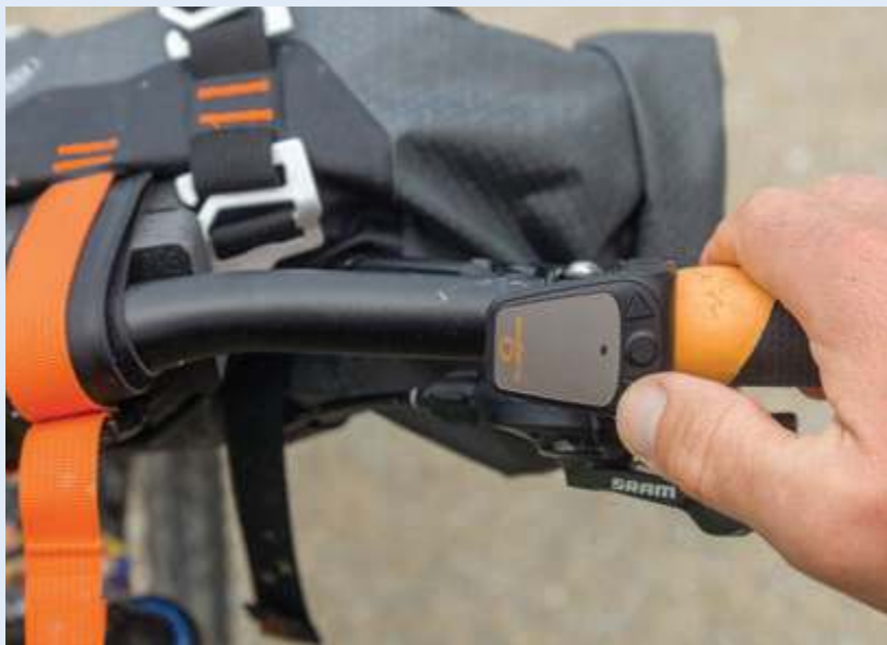
A simple wireless remote controls the Usee.
