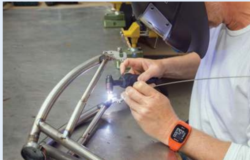
Thomas Bernds believes in doing as much production in-house as possible. Here he welds a steel frame for a 20-inch folding Bernds Bike.
