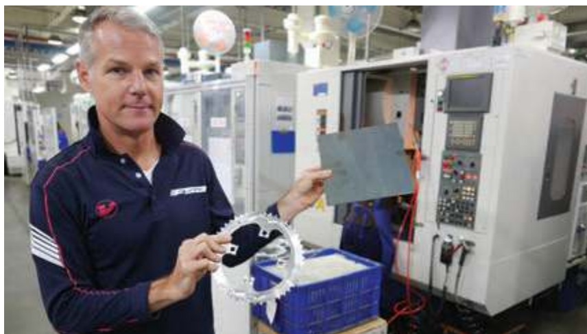
FSA's Mark Vandermolten displays an aluminum plate (right) that is about to be transformed into a chainring like the one in his other hand. (Photo:JB)
