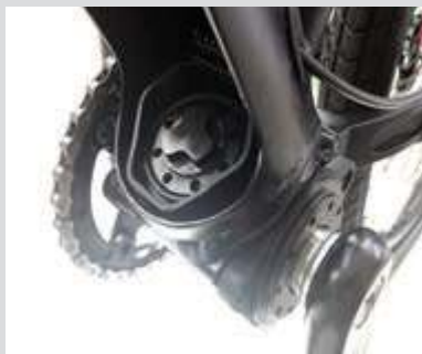
The Fazua motor sits just above the bottom bracket.
