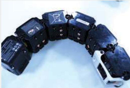
Five of the six units in the Snake Pack contain battery cells, and the sixth holds the battery management system that controls the batteries.
