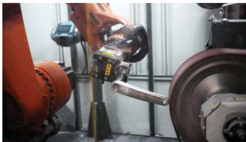
Robots at Miranda's Agueda, Portugal factory polish cranks.
