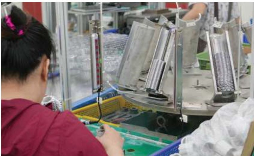
Making cassettes for SRAM's newest 1x drivetrain, Eagle
