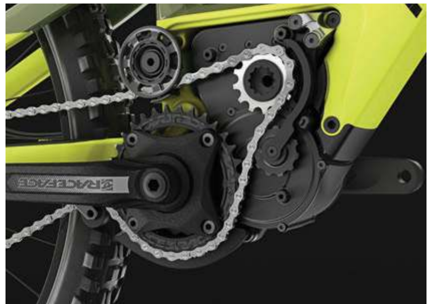
Rocky Mountain developed its own mid-drive system for the Altitude Powerplay e-mountain bike.
