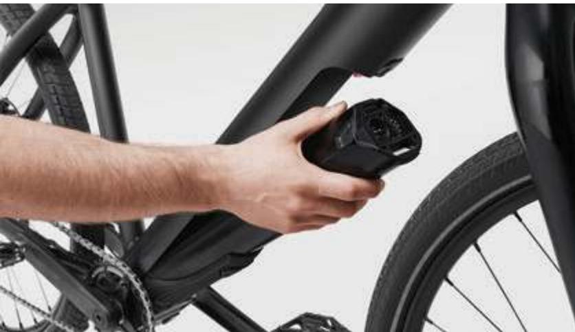
The motor and battery pack for the Fazua Evation drive can be removed from the bike.
