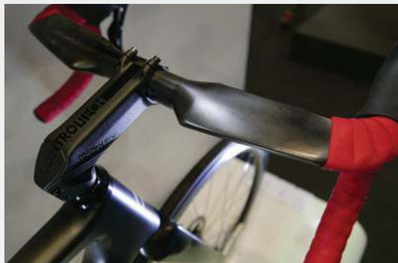
Brake and shifting cables run through tiny holes in the fork and then through the stem, fork and frame for a very clean look. (Photo: JB)
