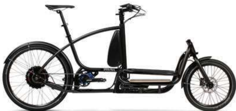
Douze e-cargo bike with GoSwiss rear hub motor and Pinion gearbox
