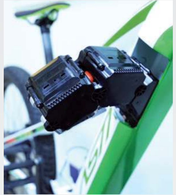
The Snake Battery System consists of hinged pieces that can be easily installed or removed from the frame.
