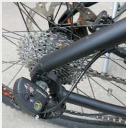
SRAM combines a rear derailleur with an internal gear hub for a gear range of 610 percent.
