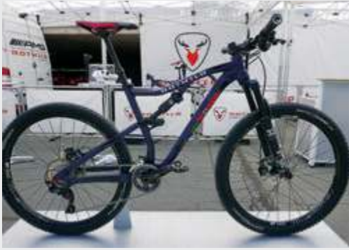
The new Rotwild R.C1 FS cross-country bike comes with or without a Brose mid-drive motor. (Photo: JB)
