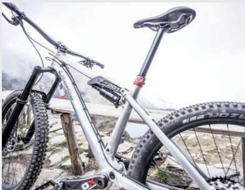
The Eightpins dropper post is built into the frame.
