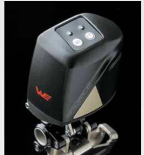
The K-Force WE front derailer houses the system's digital control box.
