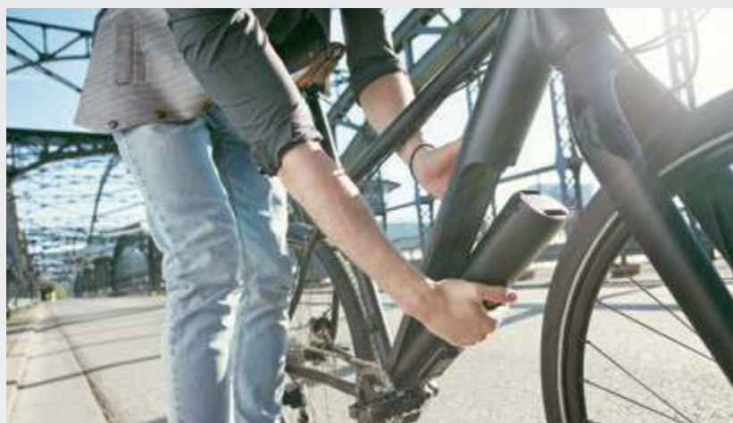
The Fazua Evation battery and motor detach quickly from the bike.
