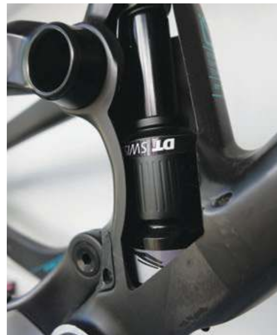
A cutaway view shows how the shock fits at the base of the seat tube.
