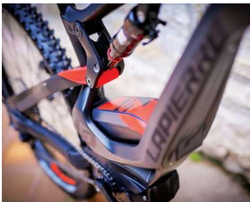
Lapierre's new Overvolt range places the battery as low as possible on the frame.
