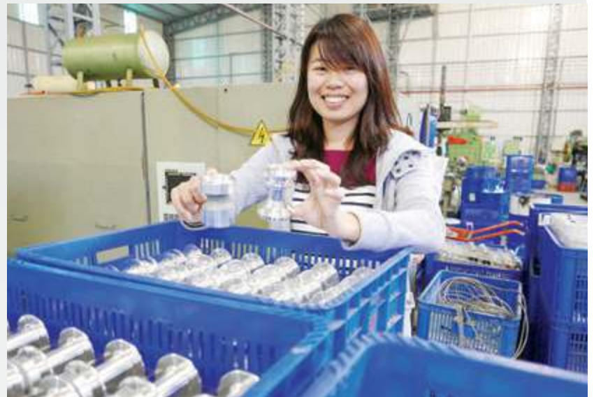
Powerway's Doris Tseng with aluminum hub shells before and after the first CNC production steps
