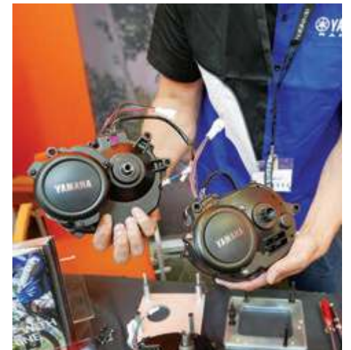
The Yamaha PW-X motor (right) is lighter and 13 percent smaller than the PW, but more powerful. (Photo: JB)
