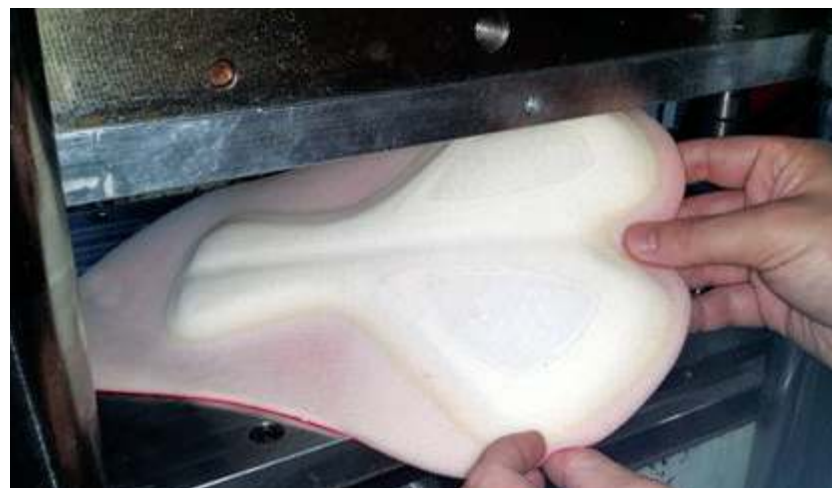
Dr Pad developed its own machinery for its Gel Injection Plus system, where liquefied silicone gel is injected directly on the open-cell foam of the pad. With the system, Dr Pad doesn't need to use adhesives or stitching to affix the gel to the pad.
