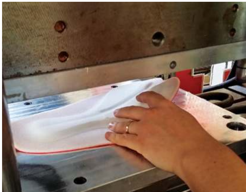
Dr Pad developed its own machinery for its Gel Injection Plus system, where liquefied silicone gel is injected directly on the open-cell foam of the pad. With the system, Dr Pad doesn't need to use adhesives or stitching to affix the gel to the pad.
