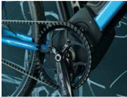
Protanium Diavelo bike with Brose motor and ContiTech belt drive
