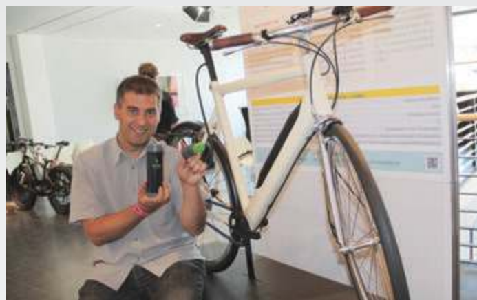
ExtraEnergy's Hannes Neupert displays the replaceable Energy Tube battery, and integrated charging cable that stores in the bike's seat tube, on the Urban Concept Bike. (Photo: JB)
