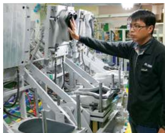
Robots on an automated vacuum and foaming carousel produce saddles 24 hours a day from 36 stations.
