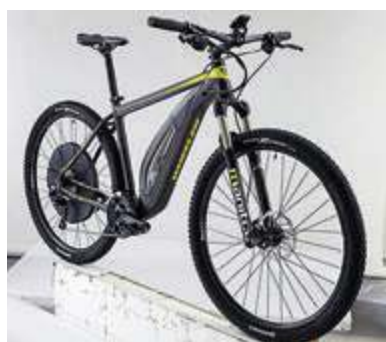
Wheeler E-Eagle with BionX D-Series motor and semi-integrated battery.
