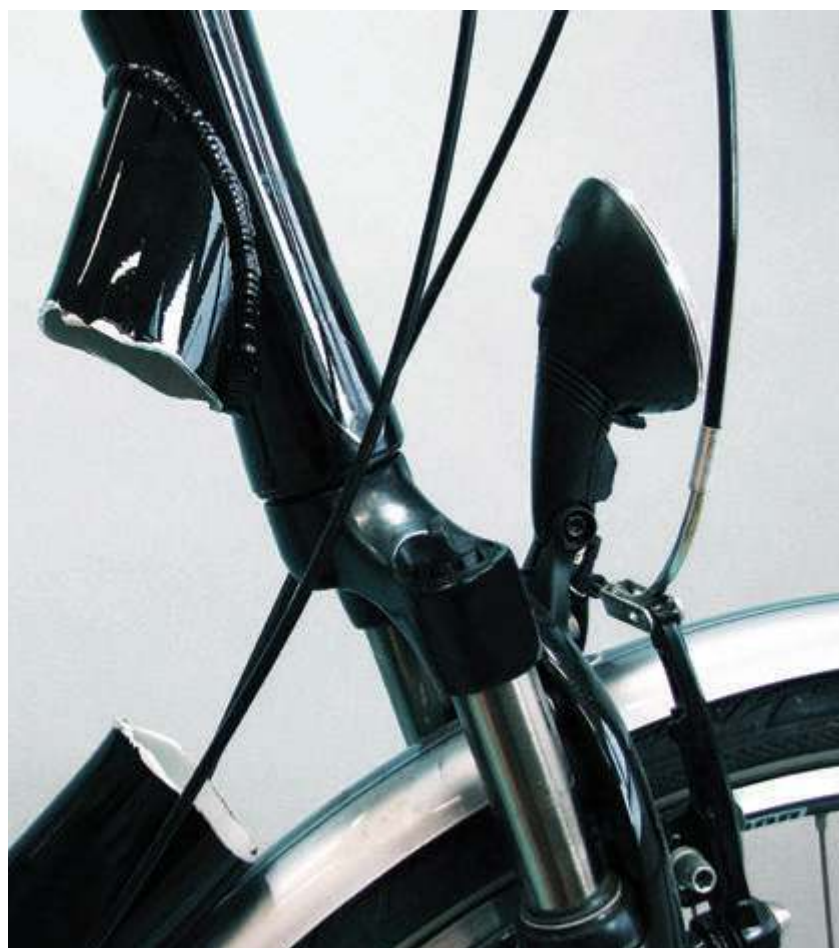
A broken frame on a step-through pedelec
