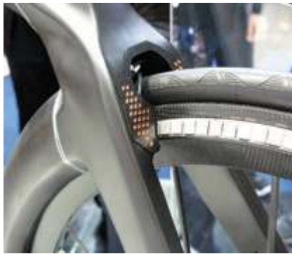
Close-up of the Velocité's rim magnets
