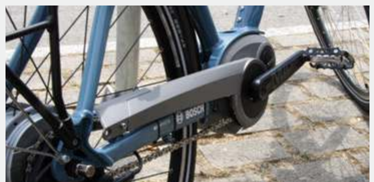
A pedelec with a Nuvinci H Sync hub and Bosch e-bike drive.
