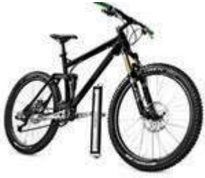
A bike with the Fazua Evation motor and battery removed.
