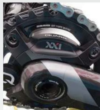
Quarq Power Meter fits SRAM 1x mountain bike drivetrains.
