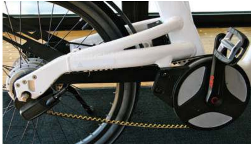
The new A2B Entz comes with an AEG e-bike system, Conti drive system and NuVinci hub. Photo: JB
