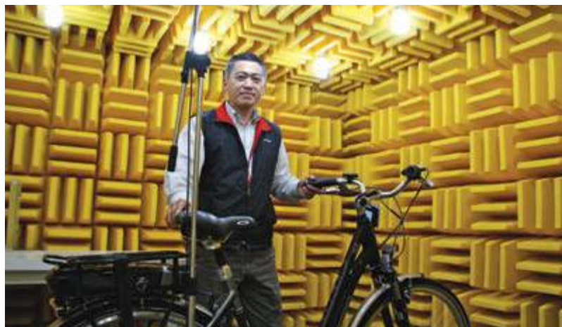
Darfon's Alou Chang tests the noise levels of the Excimer motor. (Photo:JB)
