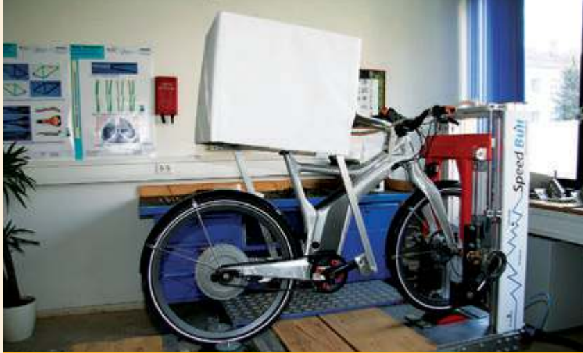
"Speed Bull" roller testing equipment is used to test bicycles, pedelecs and e-bikes.
