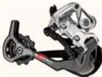
Lightweight magnesium rear derailleur has an upper jockey wheel with is offset from the cage pivot giving clearance for the 36 sprocket. © SRAM
