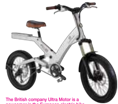
The British company Ultra Motor is a newcomer in the European electric bike market. Their A2B model involves high-end downhill components. This model with a maximum speed of 33 km/h has been developed for the US market and will be available in Europe in a similar version. (Photo: Ultra Motor)
