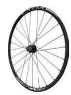
The CXD4 is for disc road and cyclocross bikes — the fastest growing category in the market. Its Equalizer offset spoke bed equalizes spoke tension on both sides of the wheel. The rims have inner and outer widths of 19mm and 24mm, respectively, and a depth of 23mm — a nice profile for shedding mud. The TRS Tubeless Ready System rim profile ensures positive bead lock with tubeless tires. Available in 700c with 6-bolt or Center-Lock disc mount.
