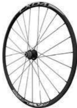
The CXD4 is for disc road and cyclocross bikes — the fastest growing category in the market. Its Equalizer offset spoke bed equalizes spoke tension on both sides of the wheel. The rims have inner and outer widths of 19mm and 24mm, respectively, and a depth of 23mm — a nice profile for shedding mud. The TRS Tubeless Ready System rim profile ensures positive bead lock with tubeless tires. Available in 700c with 6-bolt or Center-Lock disc mount. **1F/J1117**
