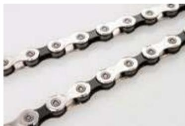
KMC's new 11-speed chain is optimized for 1x systems. Dynamic chamfer angles guide gear teeth into the chain efficiently, allowing better stability and chain retention during extreme horizontal and diagonal chain lines. Increased asymmetrical outer plate chamfer design reduces the interference of cassette gear teeth during riding, while the elongated X-Bridge improves shifting performance. **1F/J0118**
